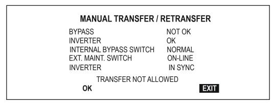
In the figure above, the message "TRANSFER NOT ALLOWED" will be flashing.
